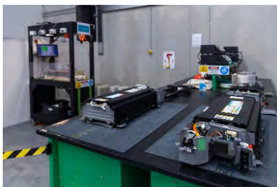
Infinitev battery testing station
