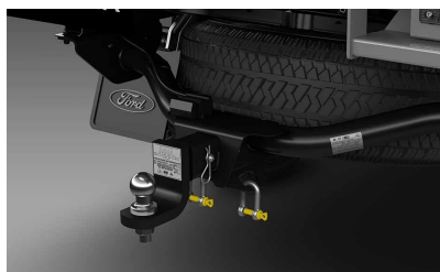
New Ford Ranger high-strength light-weight tow bar
