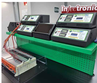
Hybrid EV battery testing station
