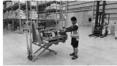
New variable height pick/pack trolleys in operation at GEL warehouse
