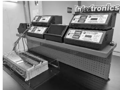
Hybrid EV battery testing station
